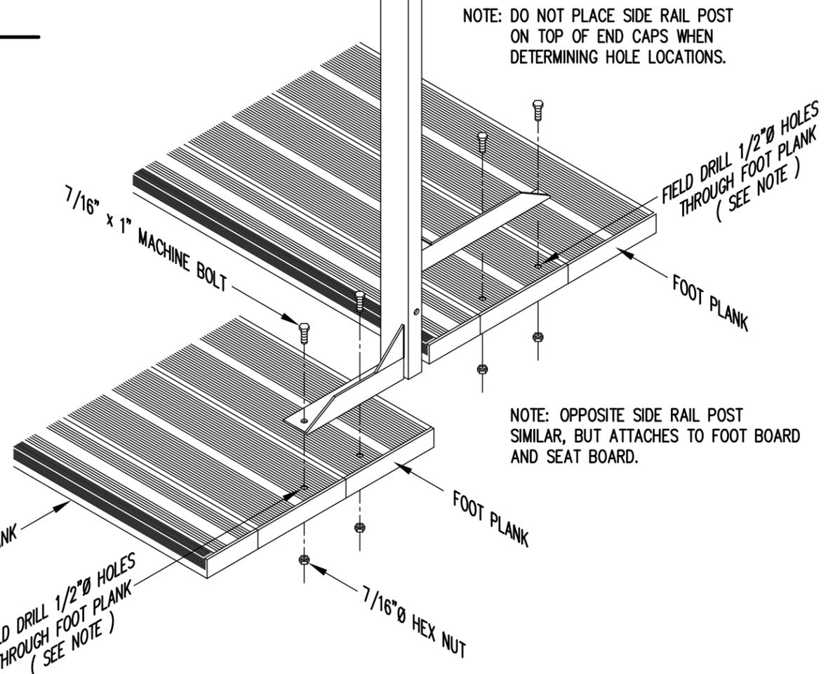
NOTE: DO NOT PLACE SIDE RAIL POST ON TOP OF END CAPS WHEN DETERMINING HOLE LOCATIONS.
