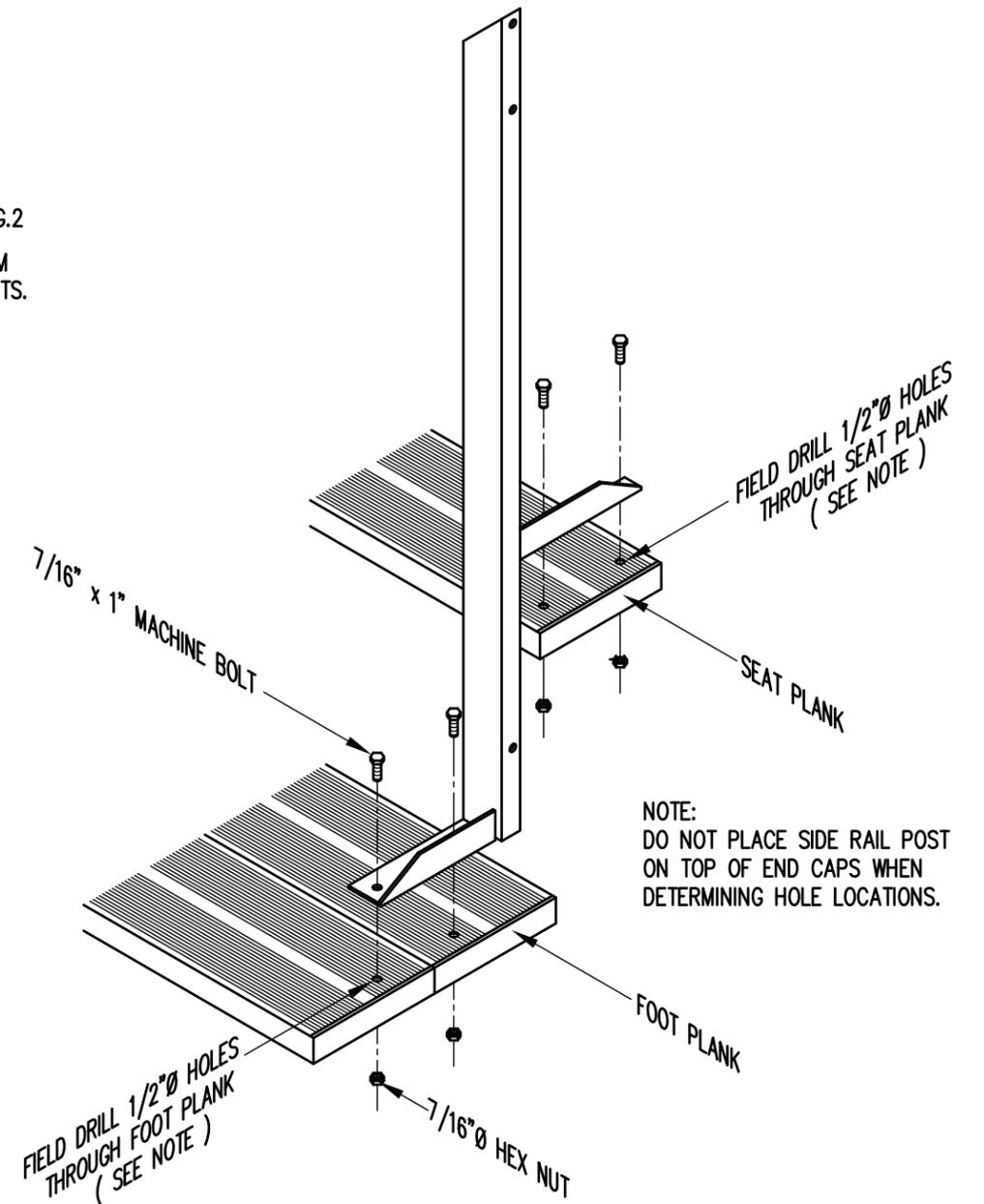
NOTE: DO NOT PLACE SIDE RAIL POST ON TOP OF END CAPS WHEN DETERMINING HOLE LOCATIONS.
